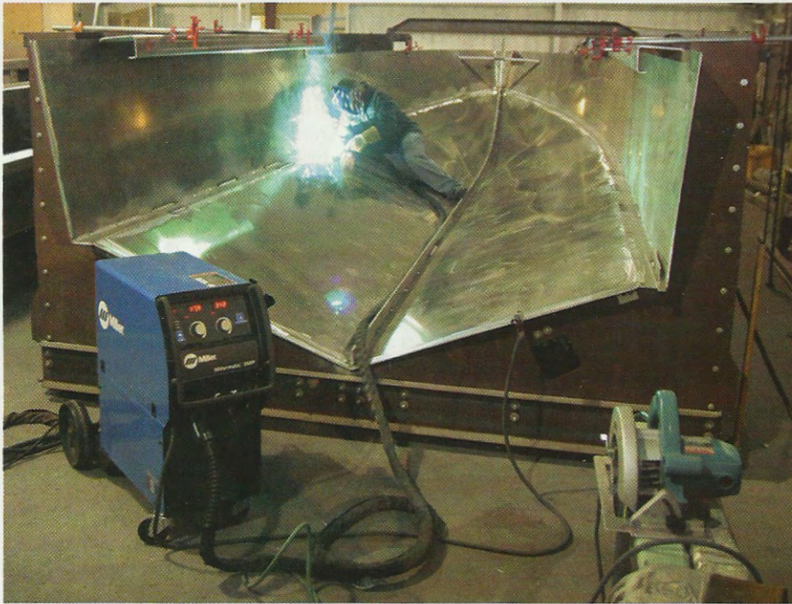
Fig. 2 — With GMAW-P, operators at Metal Shark Aluminum Boats, Jeanerette, La., can make long welds without having ribs in place because the welding process does not cause any heat-related distortion.
