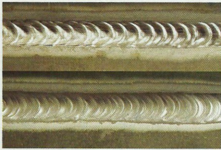
Fig. 4 — Pulsed GMAW (top) improves bead appearance and pool control so much that pulsed GMAW can substitute for AC GTAW (bottom) in many applications. Switching processes often increases travel speeds by 30% or more.
